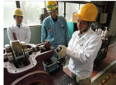
(Dismantle Kubota Pump)
