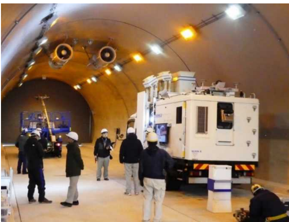
[Infrastructure Inspection and Disaster Response Robot Area] Verification of 3D tunnel inspection system
