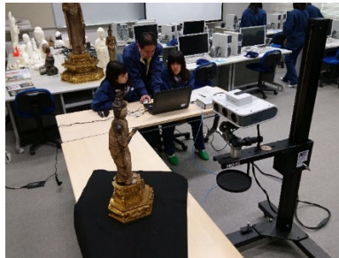
Measuring a statue using a 3D scan
